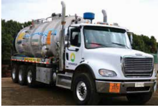
Juggler trucks enable on-board separation and dewatering to reduce waste disposal
